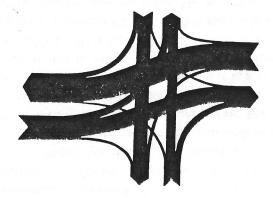
Here we have a street map with arrows of various widths on it, representing the number of vehicles per hour flowing in various directions at peak hours. In this form the diagram indicates directly what form the new intersection must take. Clearly a thick arrow requires a wide street, so that the overall pattern called for emerges directly from the diagram. It is both a requirement diagram and a form diagram. This diagram is a constructive one.
